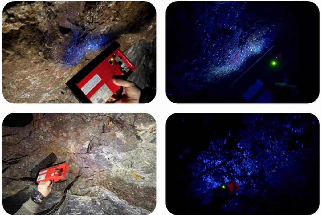
Figure 2.4.1 - Salau Underground Workings - 1230 Level Access Drives and Scheelite under UV Light (per AON Corporate Presentation, Feb 2026)
