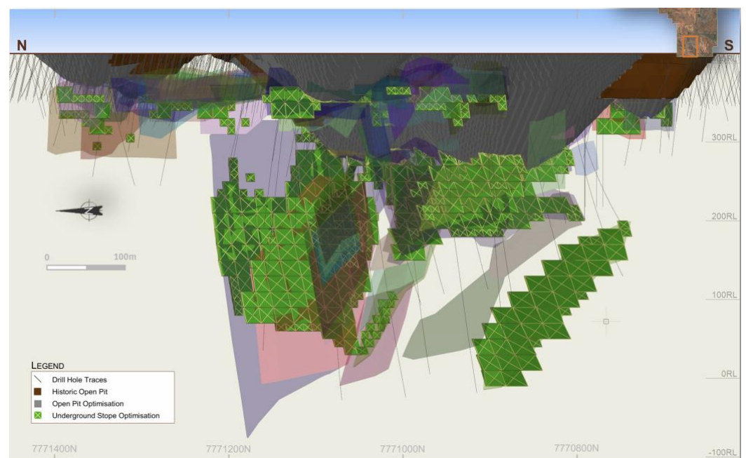
Figure 3.3.1 — Jims Deposit: Long Section with MRE Wireframes
