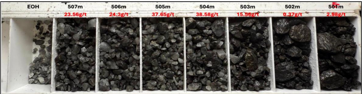
Figure 2 RC drill chips, abundant pyrrhotite, sulphides and quartz carbonate veins representing 7m @ 20.43 g/t gold, including 5m @ 27.93 g/t gold.
