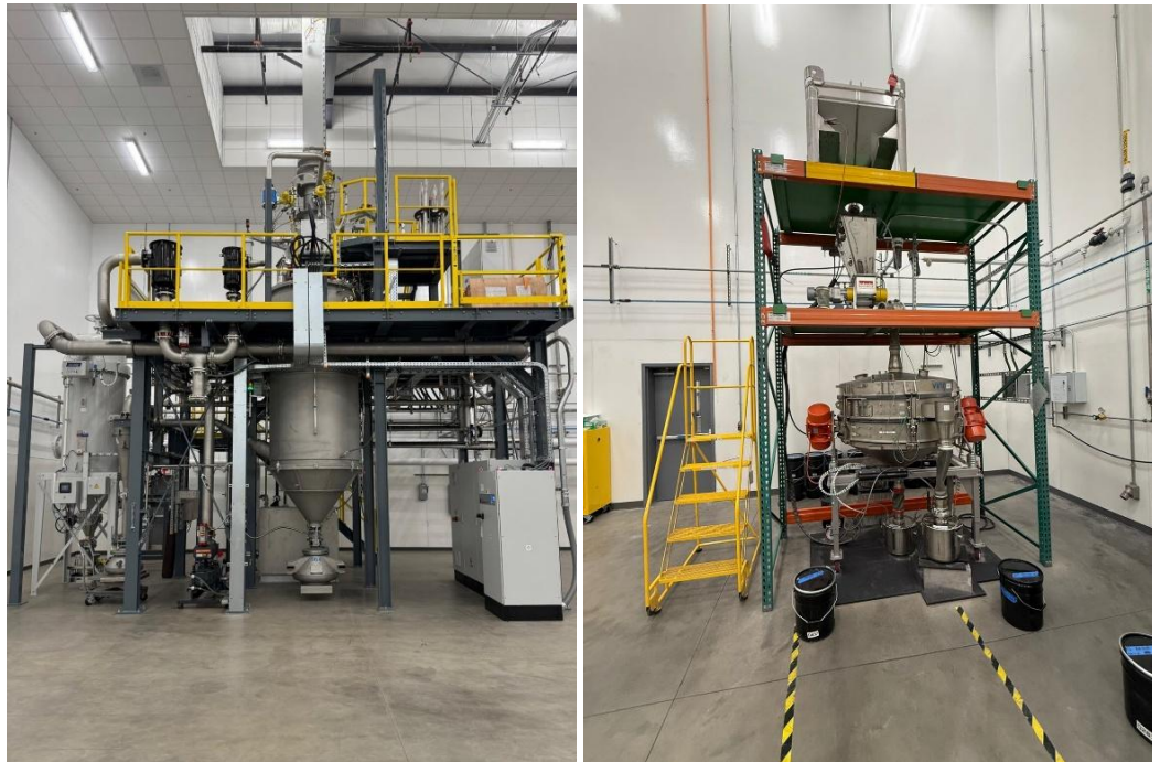
Figure 2: Commissioned Atomizer #2 and Supporting Infrastructure
