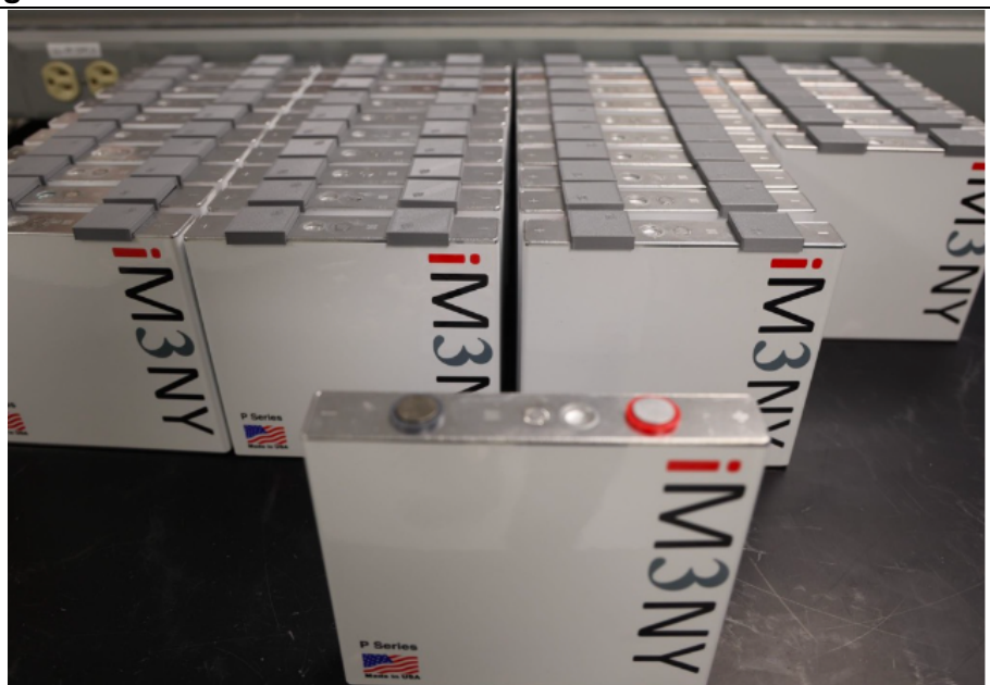
Figure 3.1 – iM2NY’s Prismatic Form Factor P series cells
